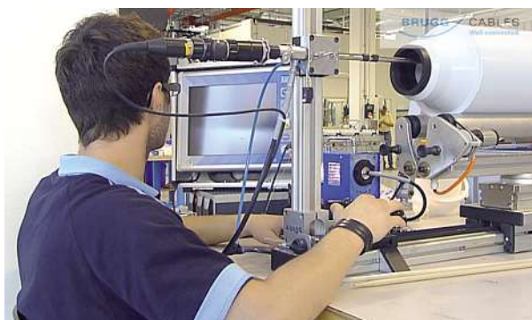
Single control of the surface of a SiR slip-on joint body after production
