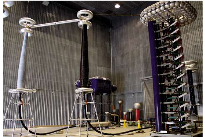
Prequalification test of 550 kV equipment
