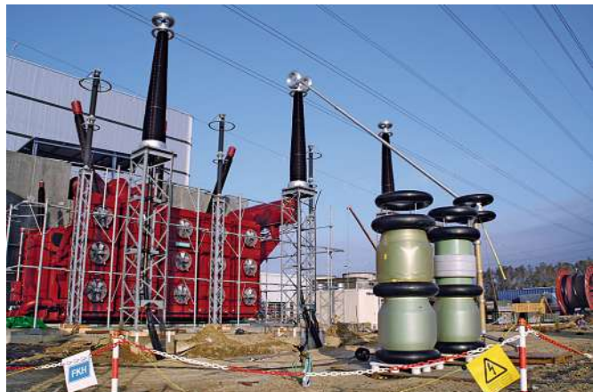
Commissioning test on-site at 420 kV porcelain terminations in Germany
