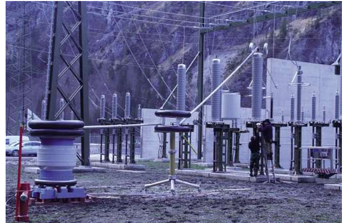
Preparation for PD measurements at terminations for a customer in Switzerland
