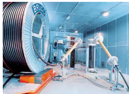
Brugg Cables' modern, fully screened test room for AC voltages up to 600 kV
