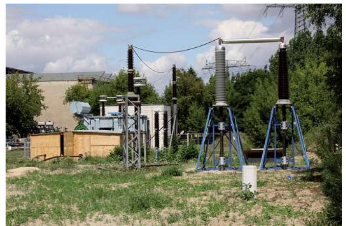
Prequalification test of 220 kV equipment at an independent test laboratory
